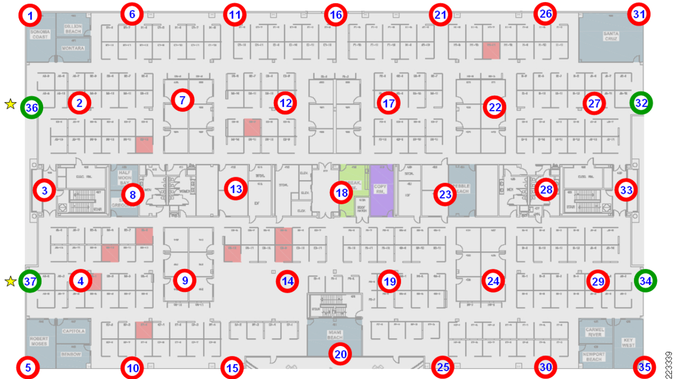
Figure 5-21 Layout for 5GHz Voice and High Speed Data, 2.4GHz Legacy, with Location
